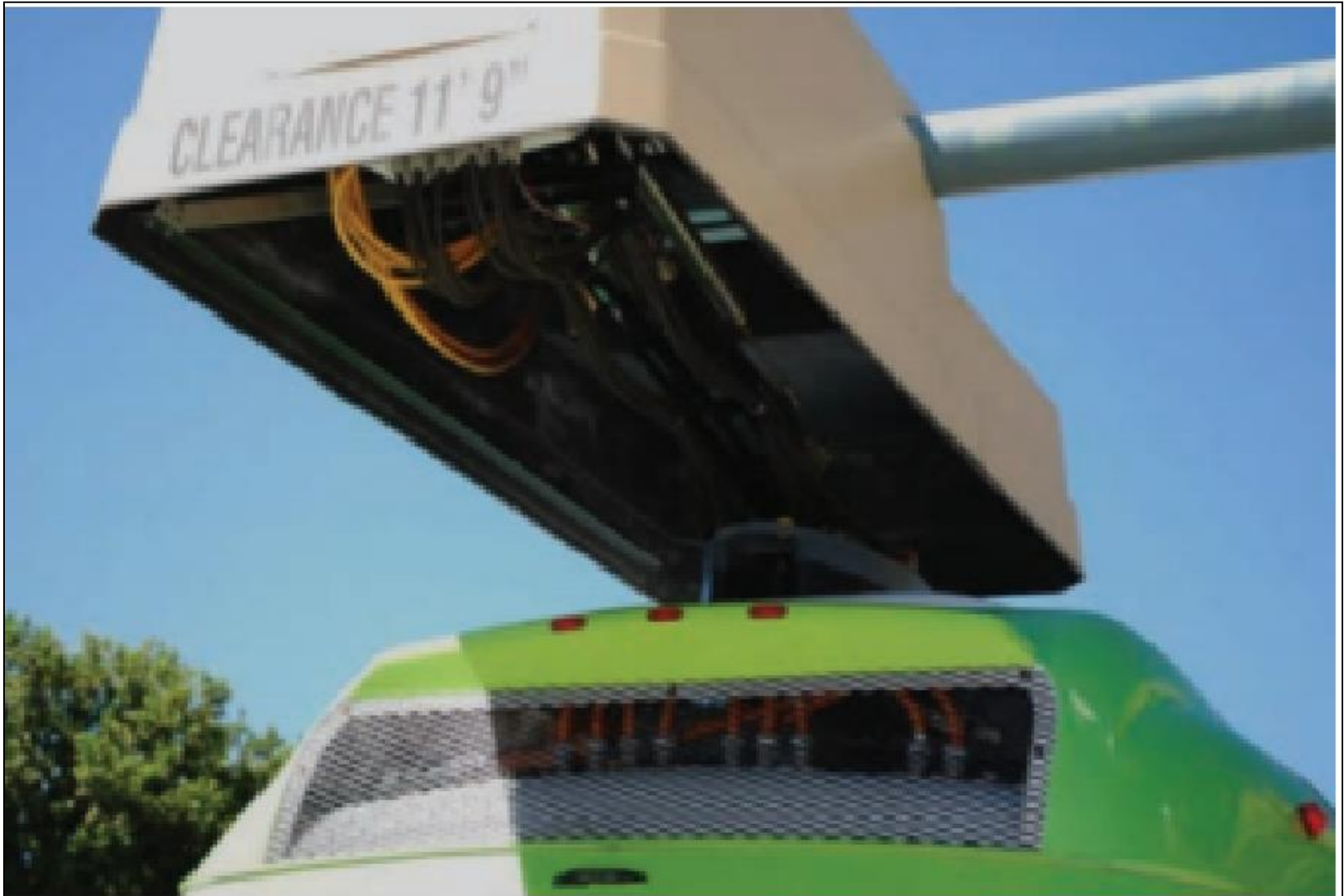
Figure 7. Foothill Transit's on-route conductive fast charger. Source: Eudy et al.
