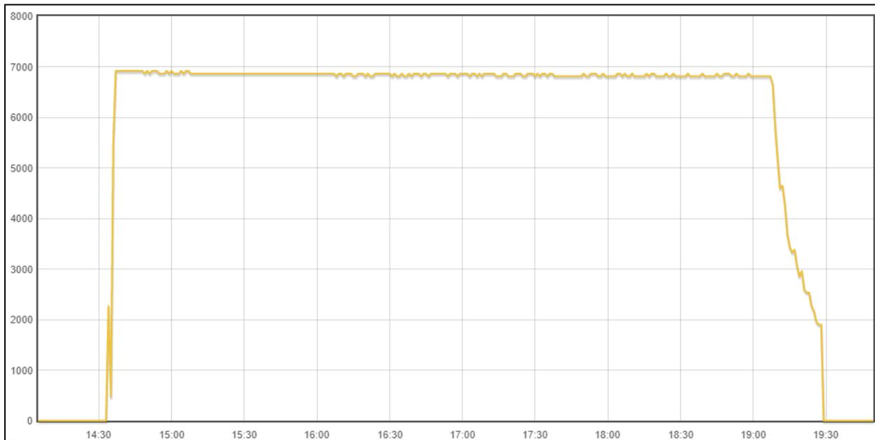
Notice that the level charging power is ~6.8 kW instead of the rated 7.2 kW because of charging losses.
