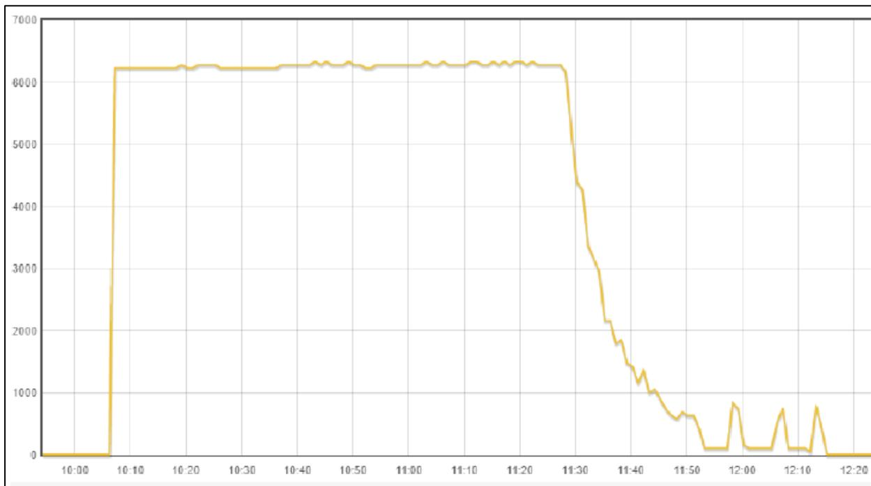
Notice that the level charging power is ~6.2 kW instead of the rated 6.6 kW because of charging losses.
