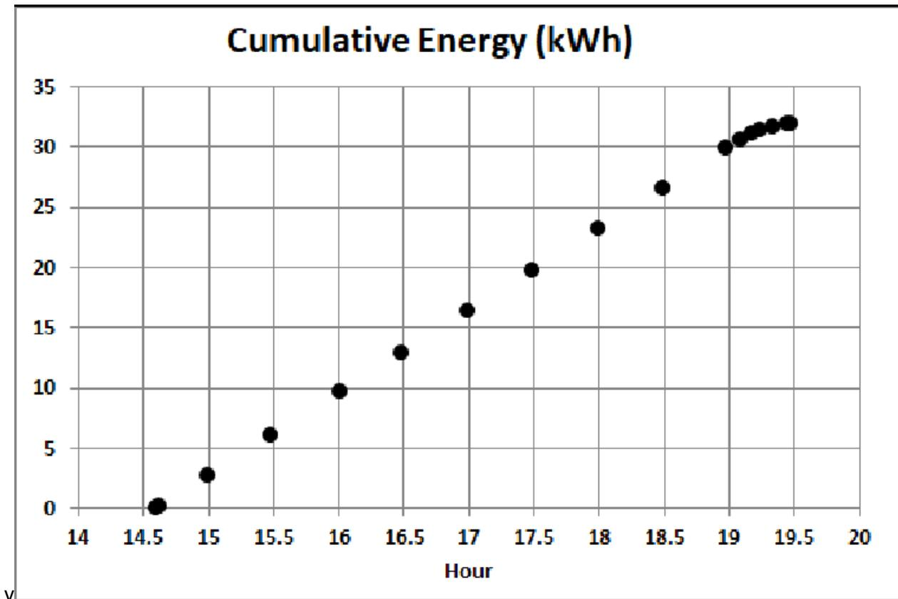
Since the power curve is nearly constant except for the last ~20 minutes of the ~5-hour charging session I conclude that the battery has several kWhs capacity beyond “100%” SOC and that the ~20-minutes slow down near the end is due to the 288 battery cells being voltage balanced.
