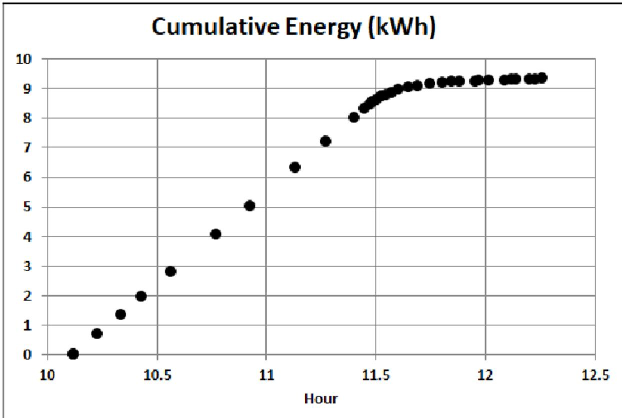
Since the power curve is nearly constant except for the last ~45 minutes of the ~5-hour charging session I conclude that the battery has several kWhs capacity beyond "100%" SOC and that the ~20-minutes jagged slow down near the end is due to the 192 battery cells being voltage balanced.
