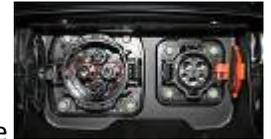
Combo combines level-2 and level-3 in one plug.) The charging receptacles on the LEAF are , with level-3 CHAdeMO on the left and SAE-J1772 on the right. Apparently, there eventually will be adapters for BEV plugs to use both “standards”. (Ref. 19) The Tesla Model S can be charged through its supplied cable to standard 120-volts outlets and with a 240-volts standard J1772 plug. Tesla has an adapter for CHAdeMO (level-3)
