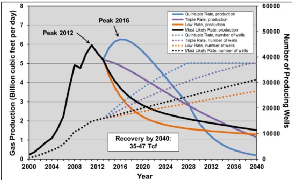
**Figure 3-25. Four drilling rate scenarios of Barnett gas production (assuming 100% of the area is drillable at eight wells per square mile).<sup>35</sup>**
