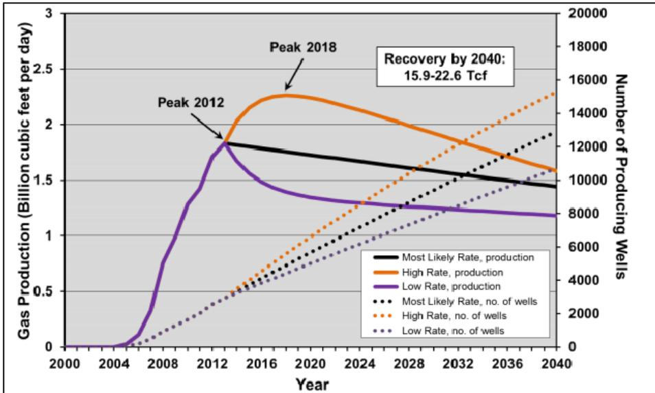
**Figure 3-78. Three drilling rate scenarios of Woodford gas production (assuming 100% of the area is drillable at 4.5 horizontal wells per square mile).<sup>119</sup>**
