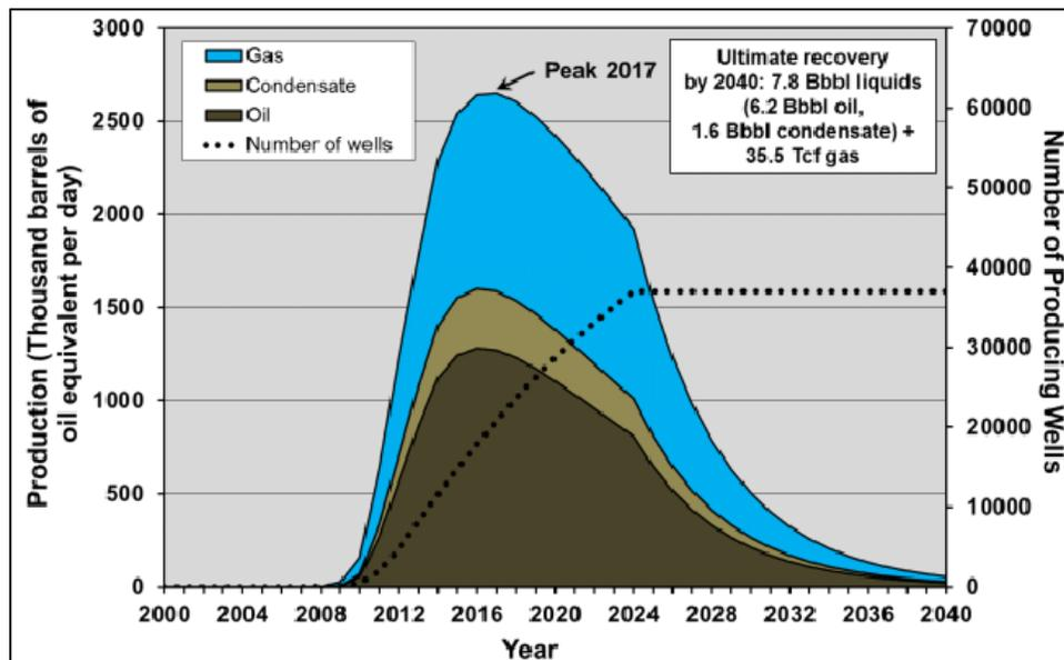
Figure 2-52. “Most Likely Rate” scenario of Eagle Ford production for oil, condensate and gas in the “Realistic Case” (80% of the remaining area is drillable at six wells per square mile).<sup>85</sup>
