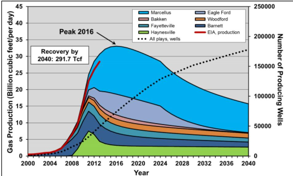
**Figure 3-115. "Most Likely Rate" scenarios for the seven shale gas plays analyzed in this report and number of producing wells, through 2040.**
