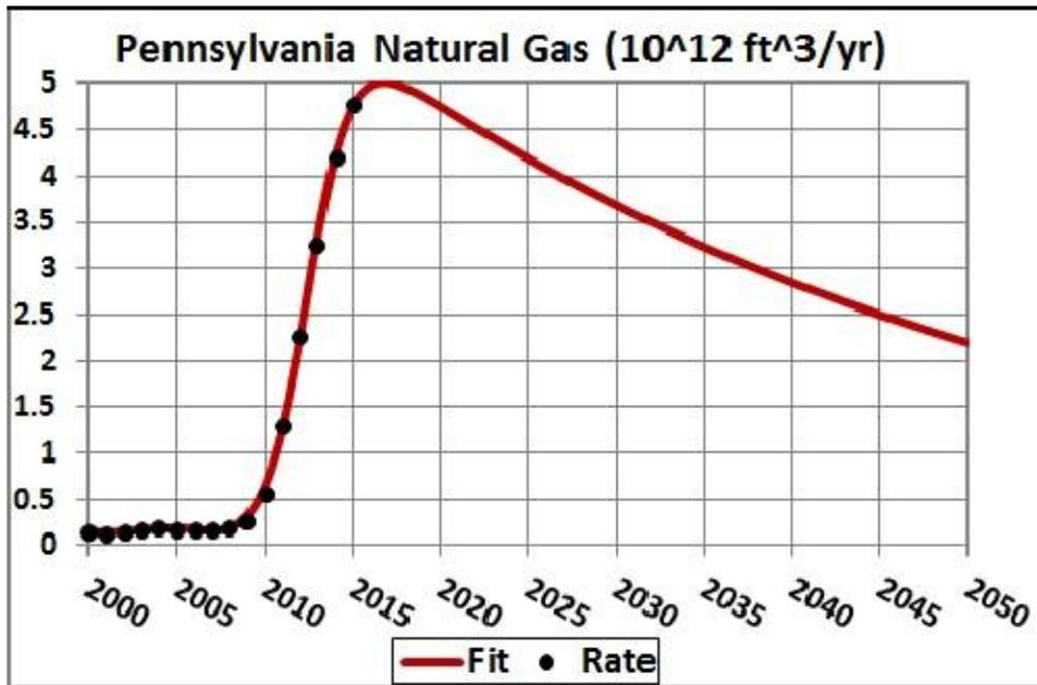
The curve has a decay exponential time constant 31.6 times the rising time constant, similar to the case for Hughes' micro-analysis for shale-gas fracking for the Marcellus play.
