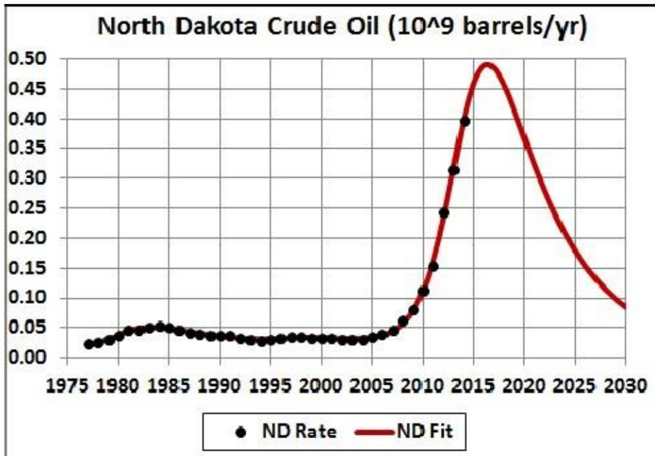
The curve has a decay exponential time constant 3.4 times the rising time constant, similar to the case for Hughes' micro-analysis for tight-oil fracking for the Bakken play.
