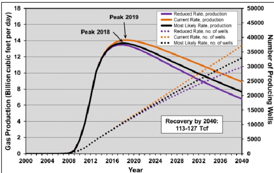
**Figure 3-98. Three drilling rate scenarios of Marcellus gas production in Pennsylvania (assuming 80% of the area is drillable at 4.3 wells per square mile).<sup>148</sup>**
