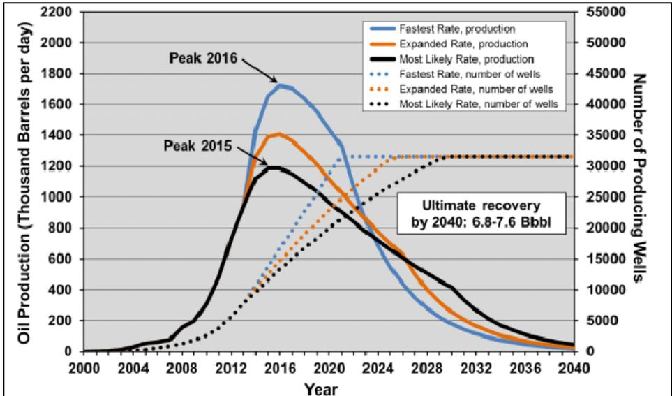
**Figure 2-26. Three drilling rate scenarios of Bakken tight oil production, in the “Realistic Case” (80% of the remaining play area is drillable at three wells per square mile).<sup>48</sup>**
