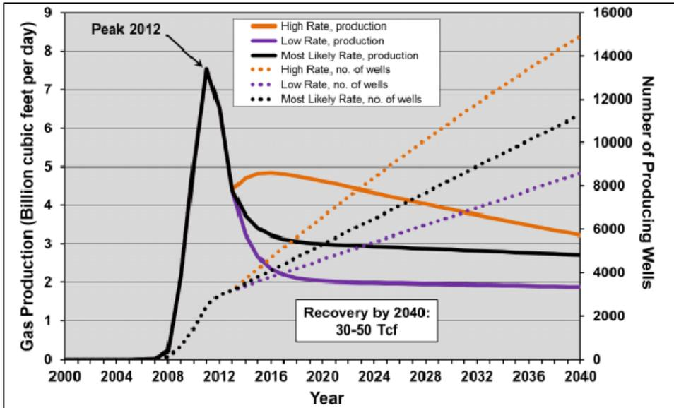
**Figure 3-43. Three drilling rate scenarios of Haynesville gas production (assuming 100% of the area is drillable at six wells per square mile).<sup>65</sup>**
