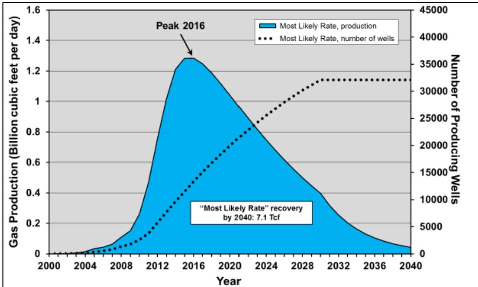
**Figure 3-112. "Most Likely Rate" scenario of Bakken gas production in the "Realistic Case" (80% of the remaining area is drillable at three wells per square mile).**
