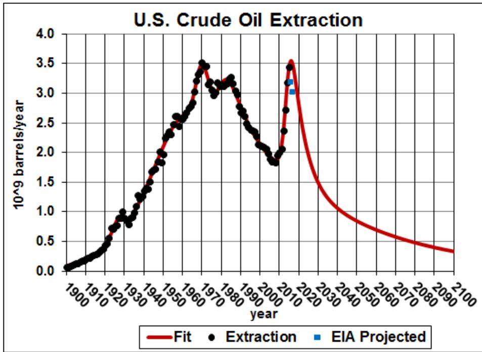
The curve's final peak has a decay exponential time constant 4.4 times the rising time constant, similar to the case for Hughes' micro-analysis for tight-oil fracking in the U.S.
