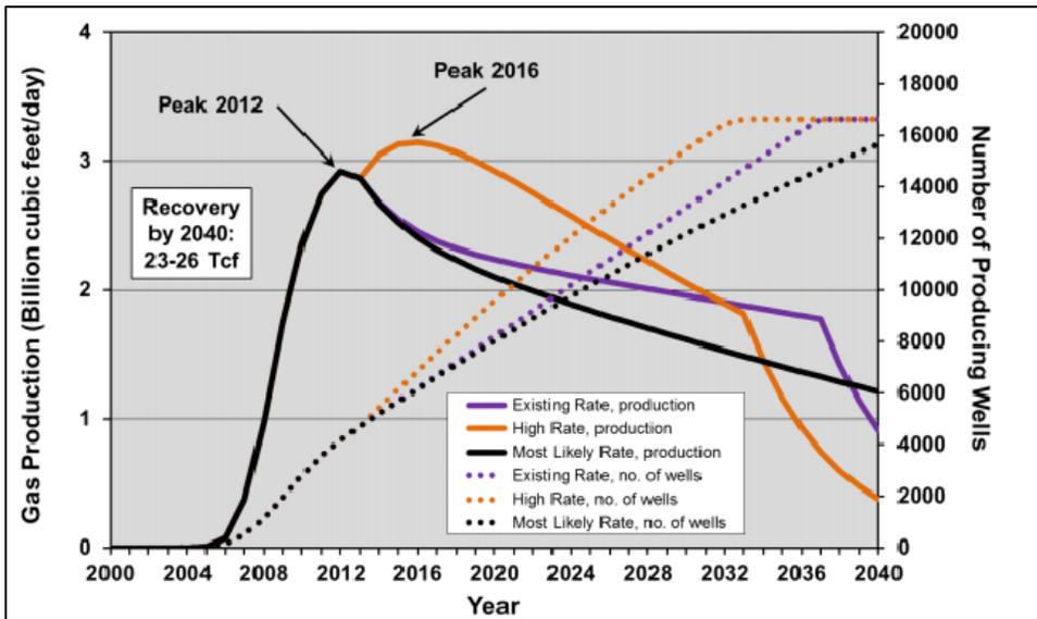
**Figure 3-59. Three drilling rate scenarios of Fayetteville gas production (assuming 100% of the area is drillable eight wells per square mile).<sup>90</sup>**
