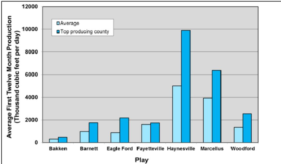
**Figure 1-5. Average first-year gas production per well in 2013 from horizontal wells both play-wide and in the top-producing county for the plays analyzed in this report.<sup>9</sup>**
