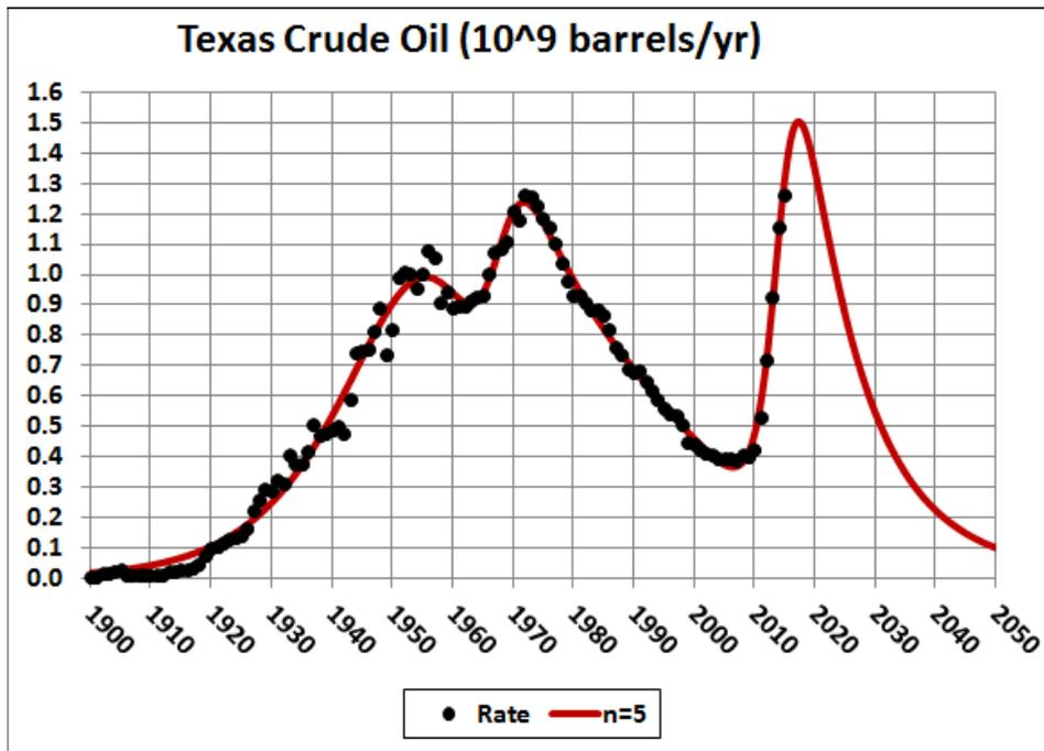
The curve's final peak has a decay exponential time constant 5 times the rising time constant, similar to the case for Hughes' micro-analysis for tight-oil fracking for the Eagle Ford play.
