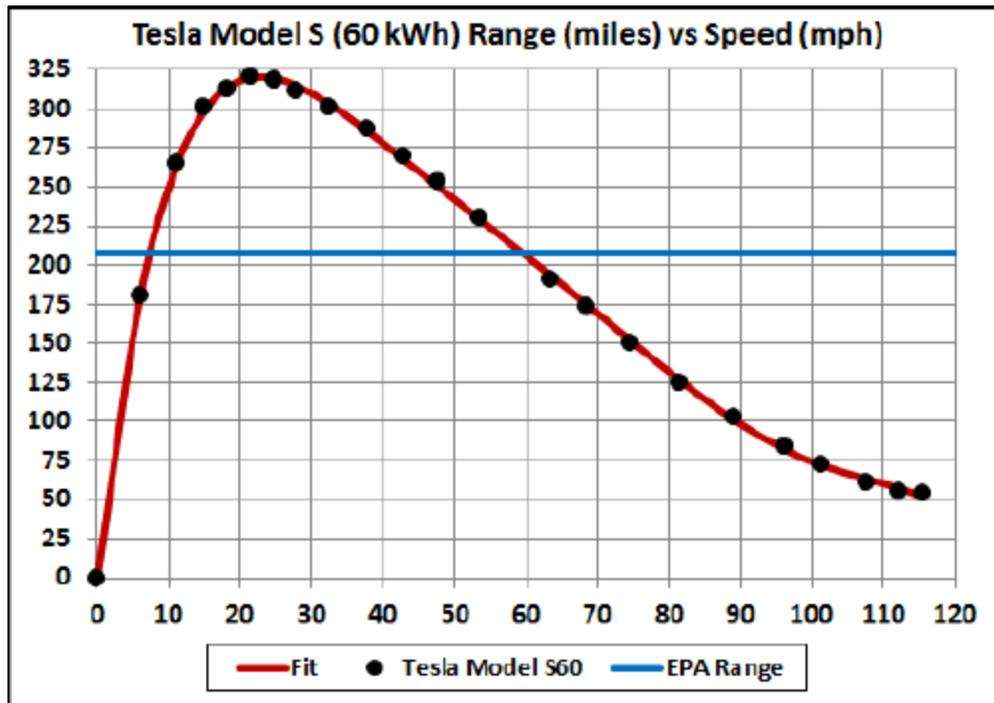
The red curve in this graph is the  $670.5 \cdot \tanh(s/21.35 \text{ miles}) \cdot \exp(s/48.16)$  (s in mph) fit to the Tesla Model S range vs speed data.
