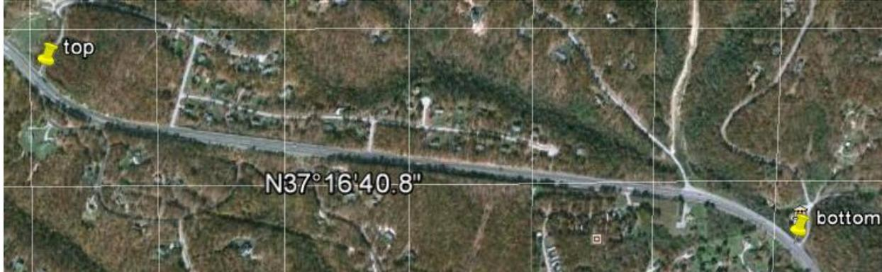
The elevation change was 456 ft = 139 meters. The speed was constant at 55 mph = 24.6 m/s and there was no wind. The slope % =  $100 \cdot 139 / 2043 = 6.8\%$ . Temperature was 70 deg F.
