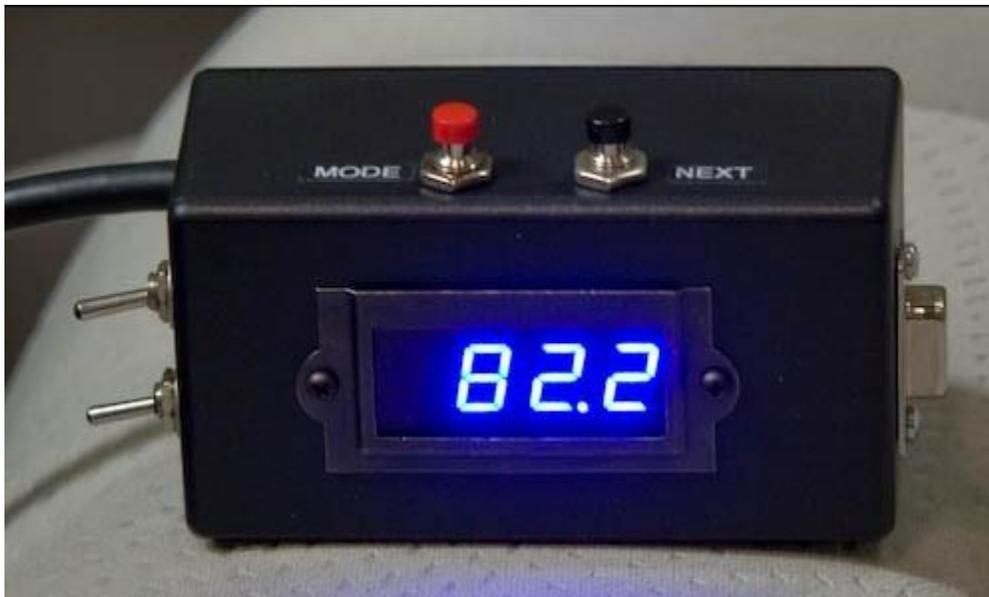
It attaches to the OBD2 plug under the dash.
