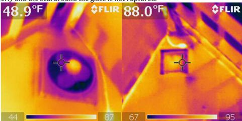
The first picture is the west window, the second picture is the east window. We later discovered that the west window was not fully closing because the window latch was not fully latched open.
