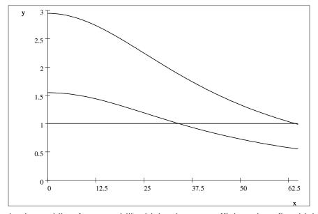
Above the horizontal line for r = 1 hilly driving is more efficient than flat driving.
