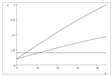
Above the horizontal line for r=1 hilly driving is more efficient than flat driving. Ratio versus vehicle speed (mph) for hill angles 20 degrees and 10 degrees (lower curve):
