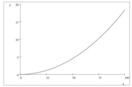
Here is a plot of the minimum hill angle (degrees) versus regeneration, f, going down the hill for 65 mph speed in order that hilly driving to be more efficient than flat driving:
