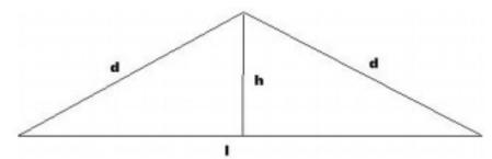
Let  $d = \text{sides of the triangle and } l = \text{the base of the triangle. Then } h = \frac{l}{2} \tan \theta = d \sin \theta$  the perpendicular distance of the peak to the base.
