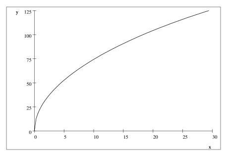
Here is a plot of the maximum vehicle speed (mph) versus fraction of regeneration, f, going down the hill for a hill angle of 20 degrees in order that hilly driving to be more efficient than flat driving:
