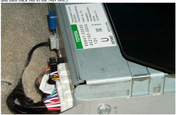
The next two pictures show the cables plugged into the CAN-View. The black cable has the small white plug on the other end to plug into the Nav box. The cable with the narrow and long white plug at the MDF port on the CAN-View box has a small white plug on the other end that attaches to the cable coming from the MFD. The cable labeled CAN has the big red OBD plug on the other end.
