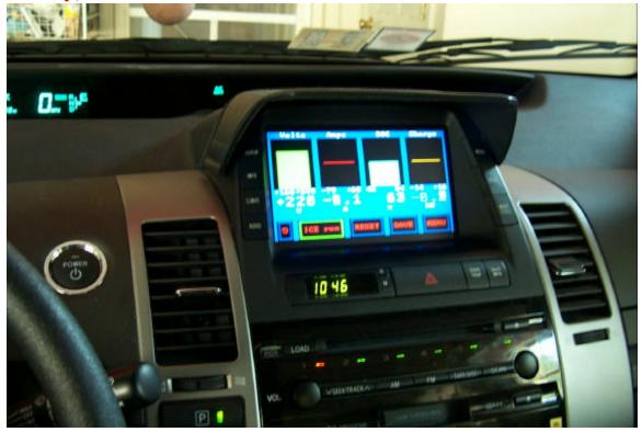
I had one small problem. When I first drove the car, the MFD gave an error screen when I put the drive selector in N or D, but the car drove ok. I think it was because the black cable was not securely attached to the CAN-View, as I later found it unplugged. The car drives fine now.
