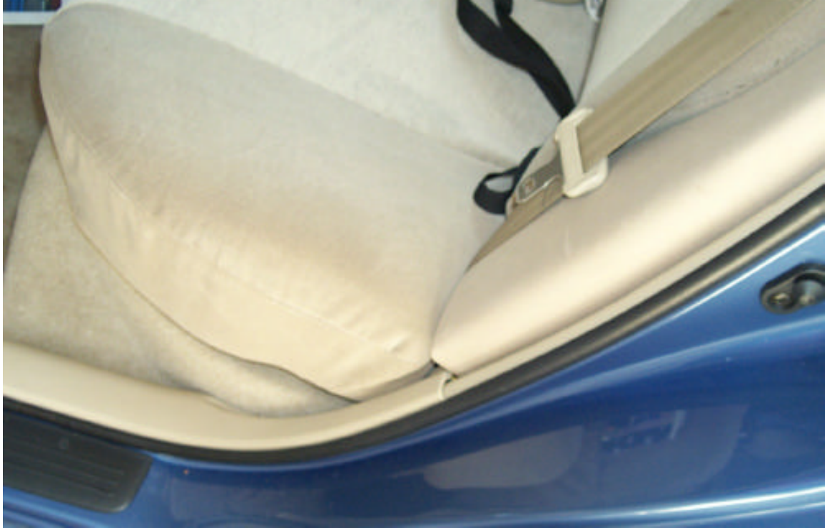
This shows the channel at the bottom and behind the back door where the wire went up.
