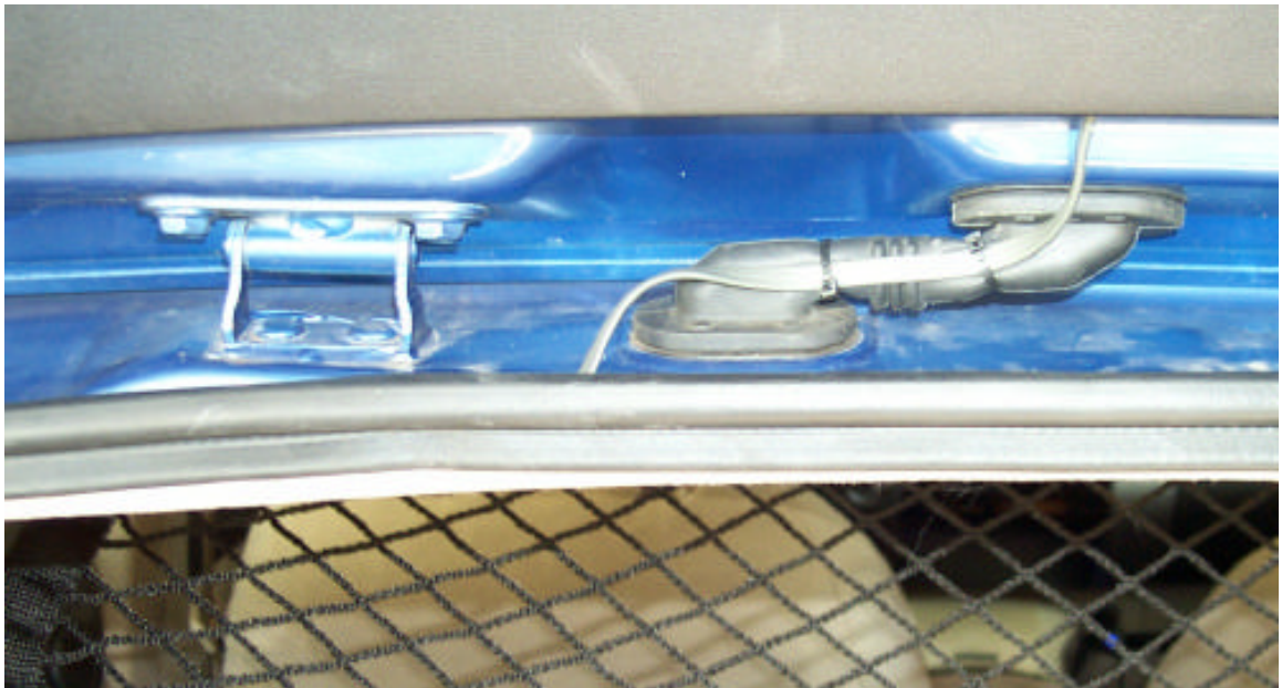
This shows how the wire went up into the hatch door after it went along under the ceiling cover.
